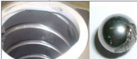
Examples of rolling contact fatigue on ballnut raceway and steel ball element.
